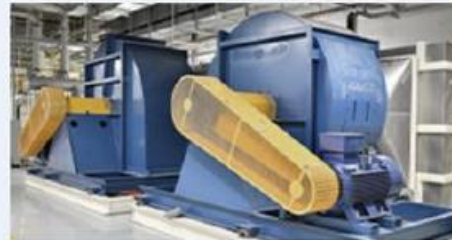
Blower Ventilation Motor
